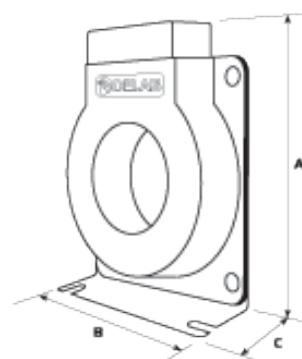
The diagram shows a side view of the Z.C.T. with three dimensions labeled: A is the height (100 mm), B is the width (50 mm), and C is the thickness (35 mm).
