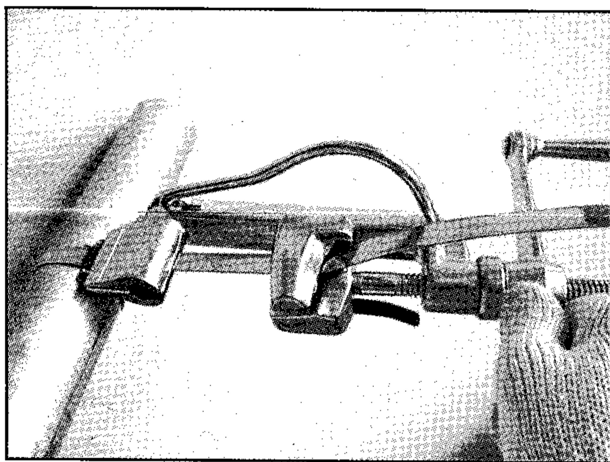
When desired tension is reached, swing tool over buckle. This movement increase tension of band and, to avoid breakage, handle must be reversed slightly as tool is swing over.
