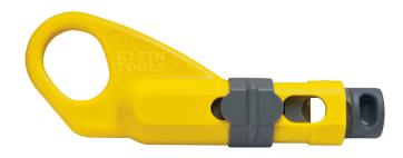
Klein Tools' Coax Combination Radial Stripper works on both standard and utility size cables. The durable, high-carbon steel cutting blades automatically adjusts to the different cable diameters. Klein's exclusive sliding depth gauge pre-measures cable for fast, accurate and repeatable stripping every time.
