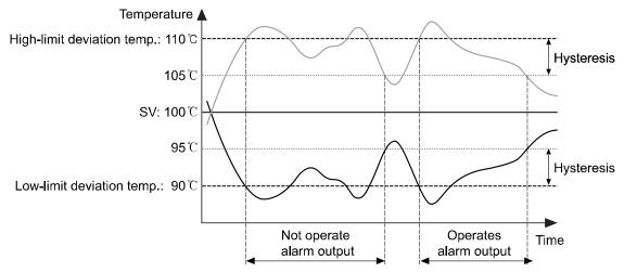
When first alarm condition occurs, alarm output does not operate. From the sencond alarm condition, alarm output operates.
