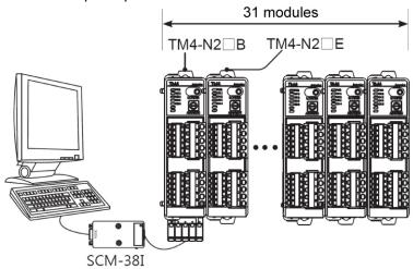
When connecting several module sets (31 modules or less), each module set requires separate power supply.
