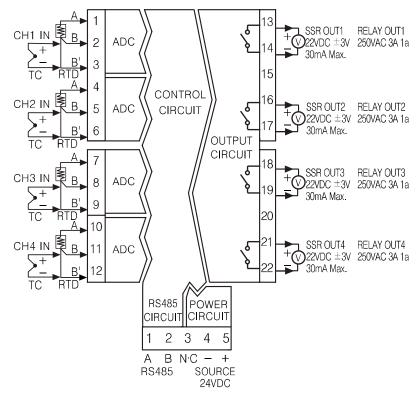
■ Power/Comm. connection terminal [Only for basic module: TM□-□□□B]
