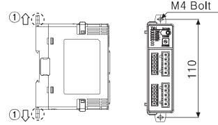
2nd Insert bolts to fix it on rail lock. (fixing torque is 0.5 to 0.9 N·m). 2 M4 Bolt
