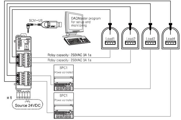
%1. Using SCM-US enables only setting parameter. To monitor and control temperature requires the additional 24VDC power supply.
