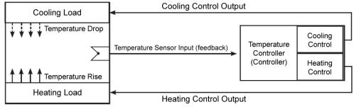
For heating/cooling control, each output for heating and cooling is automatically allocated as described in the following table.
