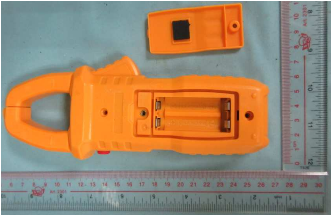
Photo 5: Battery compartment view
