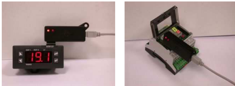
Figure 3: Inserting Memory on ATR121 (left) or DRR245 (right)
