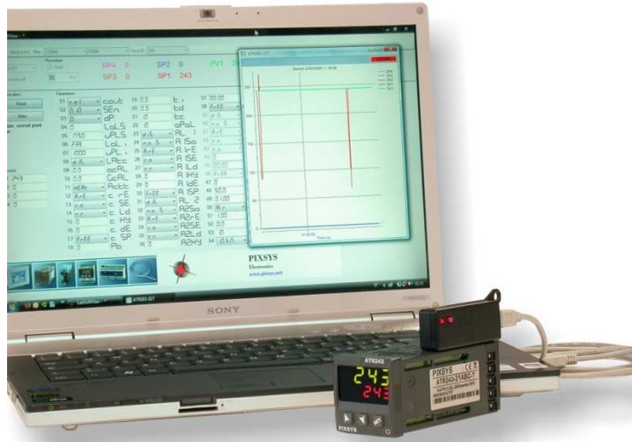
Figure 1: LabSoftView kit connecting ATR243 to a PC
